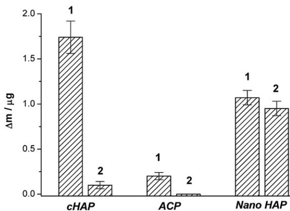
**Fig. 3** Mass change,  $\Delta m$  (= the enamel mass after treatment – the initial enamel mass), during the repair. 1: Initial adsorption state before the ultrasonic treatment. 2: After the ultrasonic treatment.
